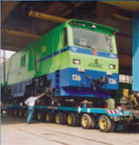
Ferrostaal's Industrial Equipment and Systems division delivered 8 electric locomotives with a weight of 130 metric tons each to transport ore in Chilean copper mines.
